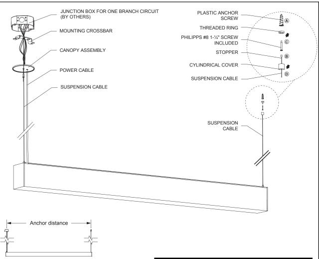
The fixtures can be manufactured in most lengths with 12" (305mm) increments. Contact the factory for precise lengths and anchoring point details.
